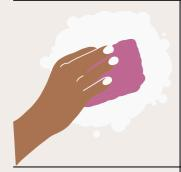
For removing superficial scratches, rub in a circular motion with a wet soft cloth and G3 compound, or similar buffing pad until the scratches are removed. Clean thoroughly with soap and water and let dry.
